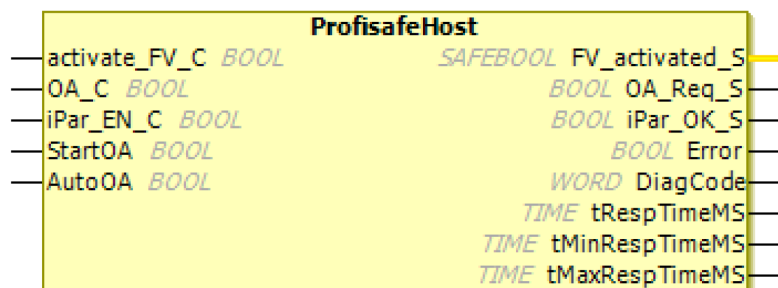
Fig. 109: Function block PROFIsafeHost
